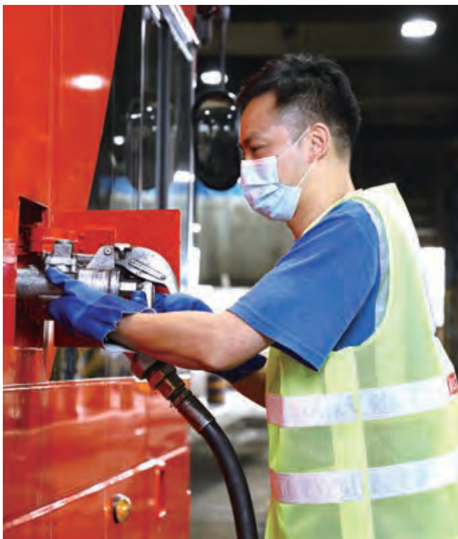
KMB and LWB's aircraft-style fuel filling system prevents spillage
