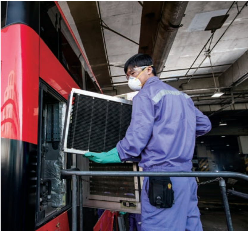
The new generation environment-friendly air-conditioning system is equipped with electronic air filters that help improve in-vehicle air quality
